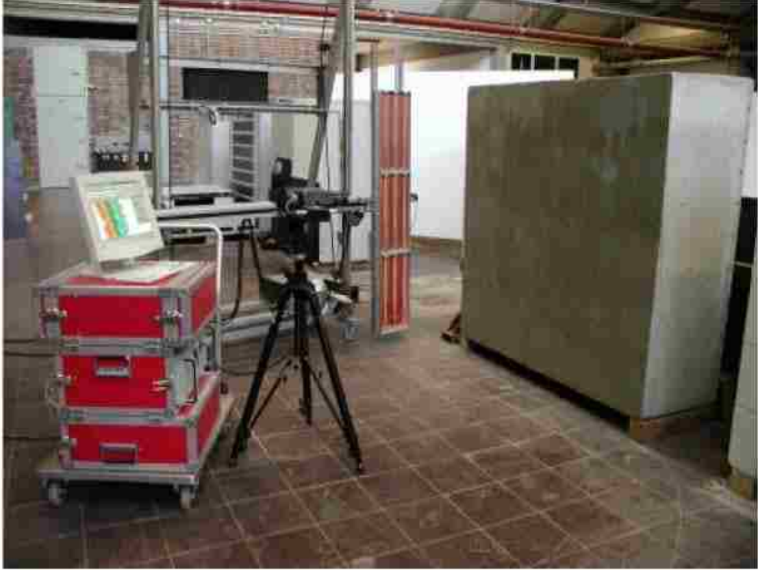
Figure 3.2: Experimental Setup of BAM experiment, including the concrete block specimen, the radiator, the infrared thermography camera and the computer unit (Wiggenhauser, Hille and Czesieki 2004)
